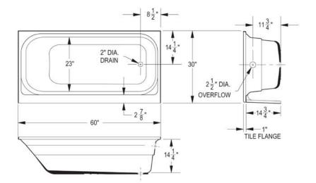
General: Furnish and install as shown on plans, TOPAZ® bathtub as manufactured by E.L. Mustee & Sons, Inc. Shall be a fiberglass 30" x 60: right hand or left hand Model \_\_\_\_\_\_. Construction shall be molded, reinforced fiberglass using matched metal molds under extreme heat and pressure. Shall meet ANSI Specification Z 124-2011. Color: \_\_\_\_\_\_ (White, Bone, Biscuit) Weight: 74 lbs. Install in compliance with local codes.
